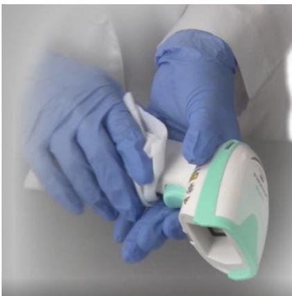
with disinfectant-ready enclosures that resist harsh chemical cleaning and embed anti-microbial additives for hospital settings where the need to suppress the growth of bacteria is always present.
